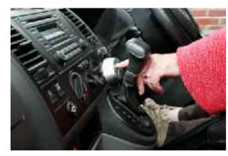
One-touch control opens door and deploys lift
