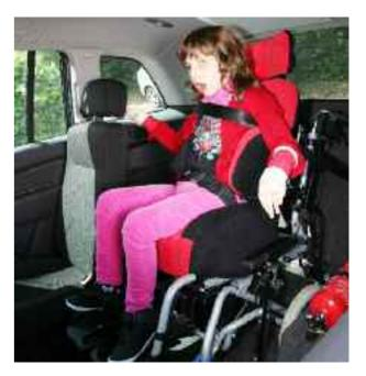
Smaller passenger WAV – room for just one, narrower, seat in the back
