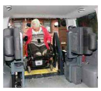
Positioning the wheelchair on the lift to exit backwards – this vehicle is fitted with folding seats in the back
