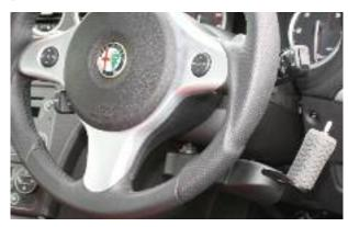
Single lever accelerator and brake – here fitted with optional indicator switch
