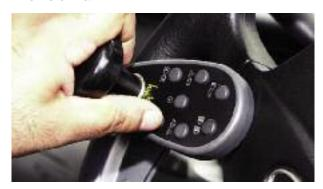
Steering knob combined with wireless secondary controls
