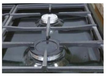
Another example of a sunken well which will capture spillages, this time on a gas hob
